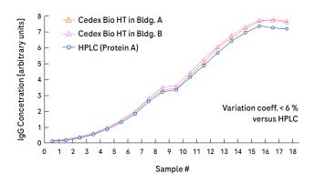
IgG: Cedex Bio HT vs HPLC: Results comparable to HPLC. The IgG titer in the culture medium was monitored over a production period of 18 days. Samples were analyzed in parallel using HPLC (Protein A) and two Cedex Bio HT Analyzers in separate locations (bldg. A/B). The consistent results represent the perfect precision and the equivalence of the methods (Roche evaluation data).
