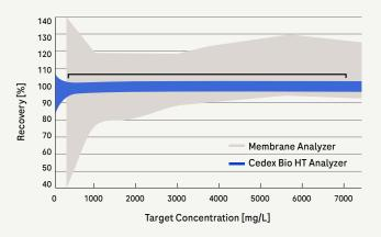
Precision in metabolite testing - comparison with membrane technology in glucose analysis: Recovery of glucose concentration was determined in parallel using the Cedex Bio HT Analyzer and a membrane analyzer (Roche evaluation data)
