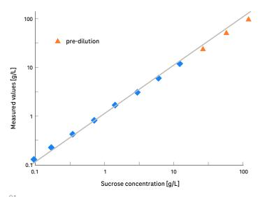
Recovery of sucrose. Sucrose was spiked into RPMI cell culture medium and measured using the Cedex Bio HT Analyzer. (Verification data of Roche Diagnostics)
