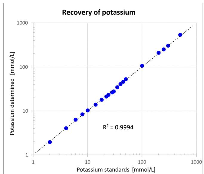
**Figure 3:** Potassium was determined in a row of standards with increasing KCl concentrations spiked to a CHO cell culture medium using the photometric potassium assay on a Cedex Bio HT Analyzer. The results show a good linearity of the test and all standards are found with deviations  $< 6\%$  from the target concentrations. (Evaluation data of Roche Diagnostics)
