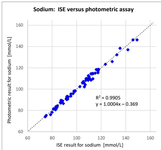
**Figure 1:** 70 samples of fermentation supernatants of various culture media were tested for sodium on a Cedex Bio HT Analyzer using the ion-selective electrode and the photometric sodium assay for comparison. The differences are all within  $\pm 4\%$ , with an average difference close to zero (ISE 0.3% higher than enzymatic), confirming the equivalence of the two methods. (Data generated with culture samples of Roche Pharma)
