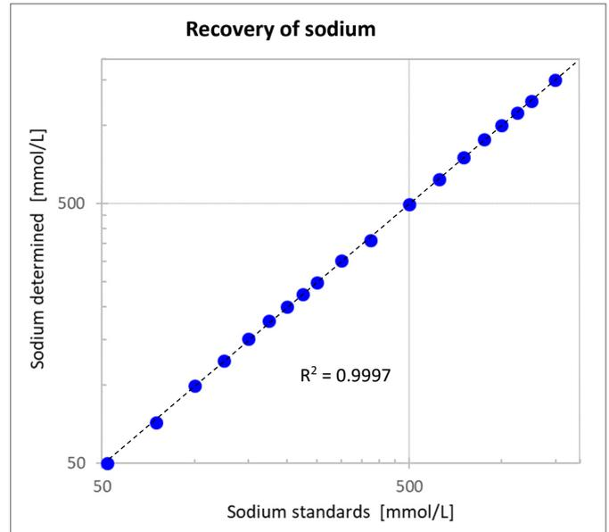
**Figure 2:** Sodium was determined in a row of standards with increasing NaCl concentrations spiked to a CHO cell culture medium using the photometric sodium assay on a Cedex Bio HT Analyzer. The results show a good linearity of the test and all standards are found with deviations  $< 2.5\%$  from the target concentrations. (Evaluation data of Roche Diagnostics)
