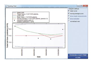
The System Suitability Test enables the user to monitor system performance via a trending chart using measurements of Density Reference Standard Beads, Control Beads and Viability Beads.
